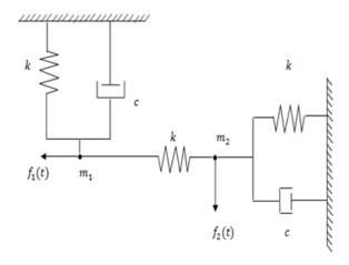
Figure 3: Model (m, k, c) of the FEEDER PAN powered by two engines
