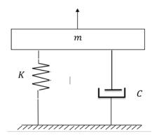
Figure 2: Model (m, k, c) of the FEEDER PAN fed by an engine
